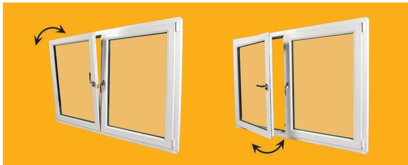
Images below show operation of Tilt & Turn windows. Left: rotate handle 180 degrees to open window in 'Tilt' state. Right: turn handle 90 degrees to fully open the window (to approx 90 degrees).
